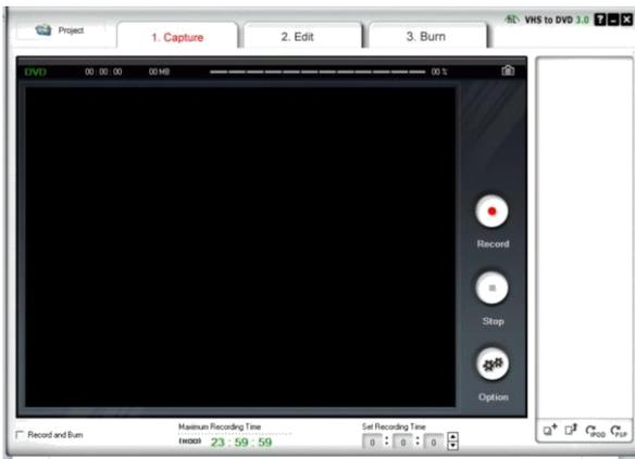
6. Once you have launched the software you will see the screen as pictured above. Connect up the capture device to the input source e.g. VHS Player, Camcorder etc, using the red, white and yellow or s-video connectors, and in the preview window you will see the live feed of your video source.
